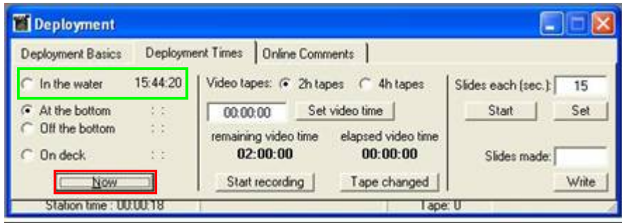
Figure 11. The deployment window that records the times that the ROV is in the water, at the bottom, off the bottom and on deck. It can also be used as a reminder when tapes need to be exchanged because the tape is full. However, this function cannot be used if tapes of other than 2 or 4 hours duration are used.
