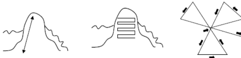
Figure 1: Common types of transect surveys. A) vertical line transect, B) grid transects and C) radial transect (Etnoyer et al. 2006, Kutti et al. 2009)
