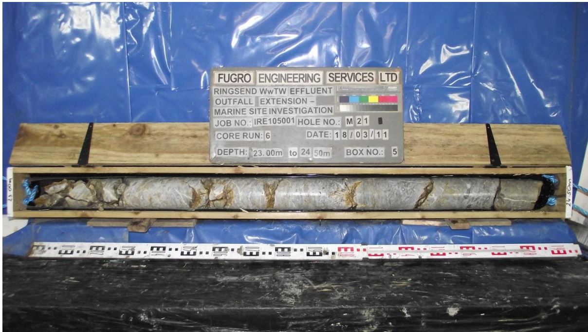
Photo 2. Core box containing a section of borehole M23.
