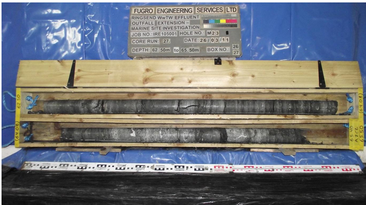
Photo 3. Core box containing a section of borehole M23.
