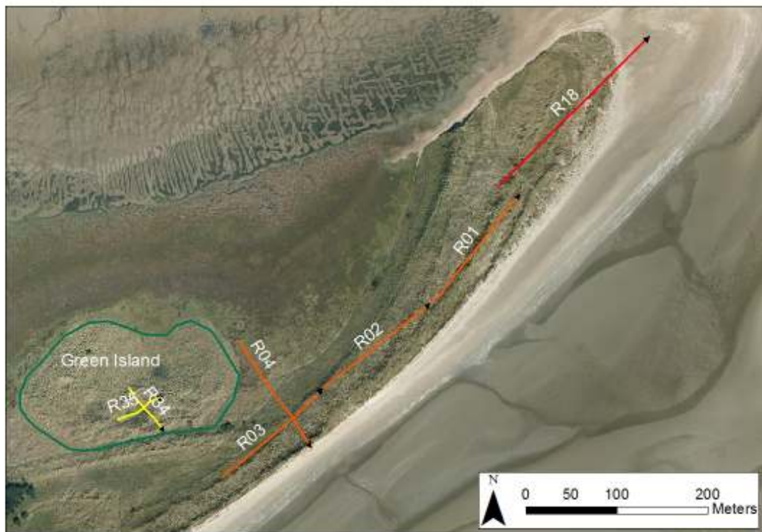
Figure 3.3 – Location of Resistivity lines with 10 m (red), 5 m (orange) and 2 m (yellow) spacing recorded in Bull Island - Site 1.
