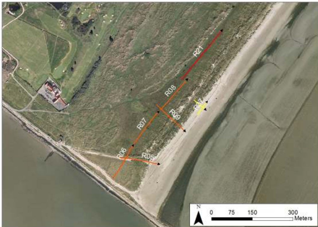
Figure 3.14 – Location of Resistivity lines with 10 m (red), 5 m (orange) and 2 m (yellow) electrode spacing recorded in Bull Island - Site 3.
