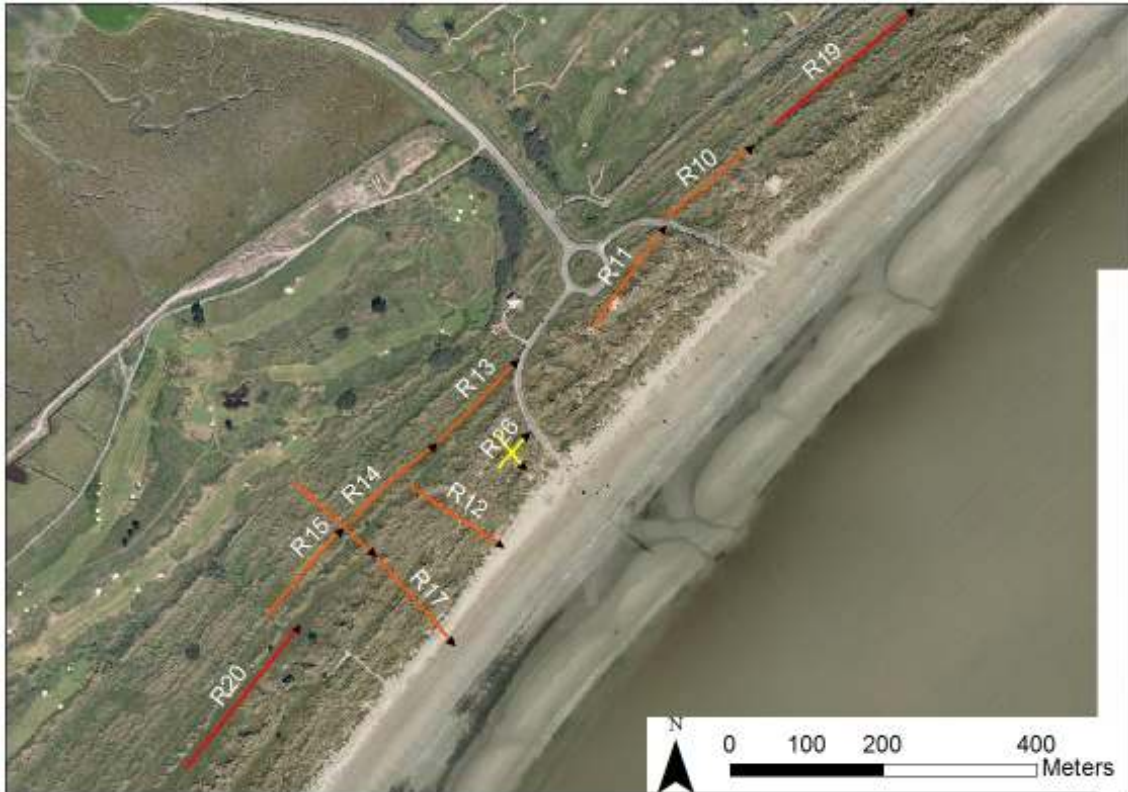
Figure 3.8 - Location of Resistivity lines with 10 m (red), 5 m (orange) and 2 m (yellow) spacing recorded in Bull Island - Site 2.
