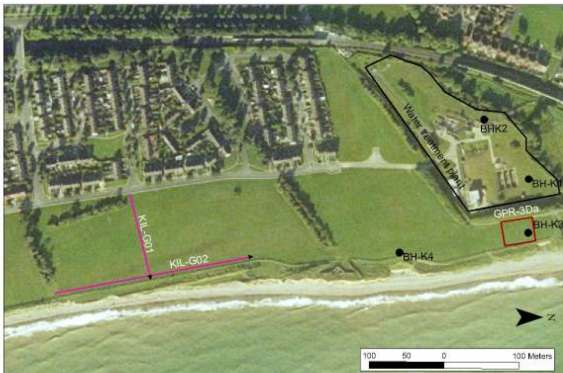
Figure 3.44 – Location of GPR profiles and 3D Model GPR-3Da collected in Killiney – Site 1.
