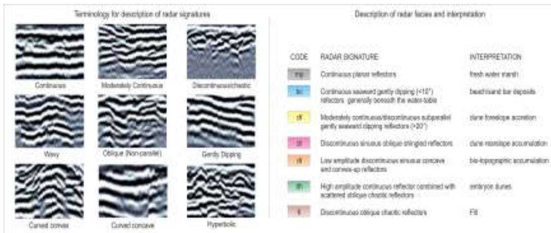
Figure 3.19 – Left – Terminology for description of radar signatures, samples shown are extracted from radargrams collected during this project. Right — colour scheme for radar facies description and interpretation modified from Bristow et al. (2000) and Neal (2004),
