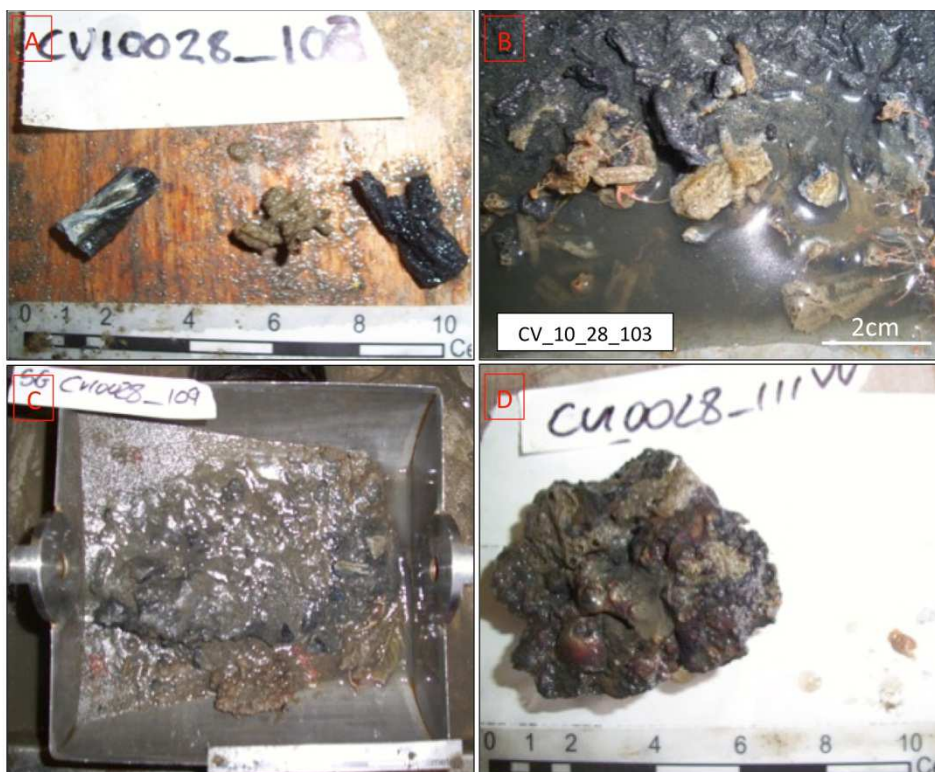
Figure 22: Grab-sampling of MDAC mound targets. (A), (B) and (C) Black anoxic sediment with high abundance of cemented fossil tube worms and MDAC (D) Large 7cm diameter carbonate nodule.
