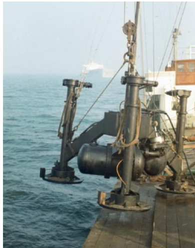
Figure 5.2: Fugro’s Seabull rig (Source: Lunne 2010)
