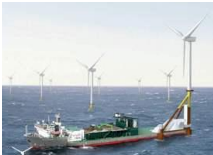
Figure 2.7: SPT Offshore Self-Installing Foundation Concept (image from sptoffshore.com)
