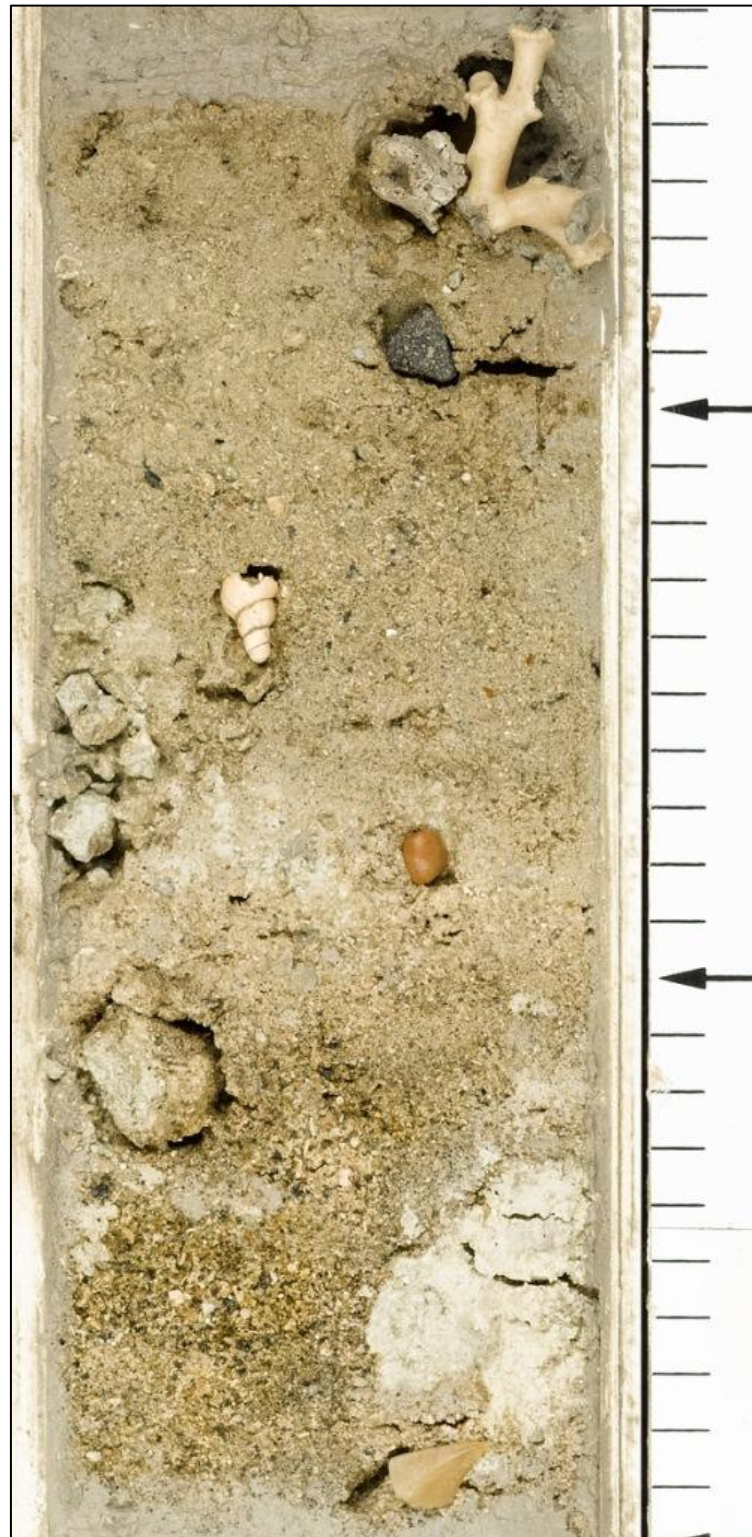
Fig.4.7.5: Coarse unit in Section 6 containing partially lithified possible biogenic rubble (middle left) and mud clasts (bright white in lower right) as well as branch size coral (a well preserved coral branch beside a heavily dissolved branch in upper right), a gastropod, and a mollusc shell (beneath mud clast) and pebbles.
