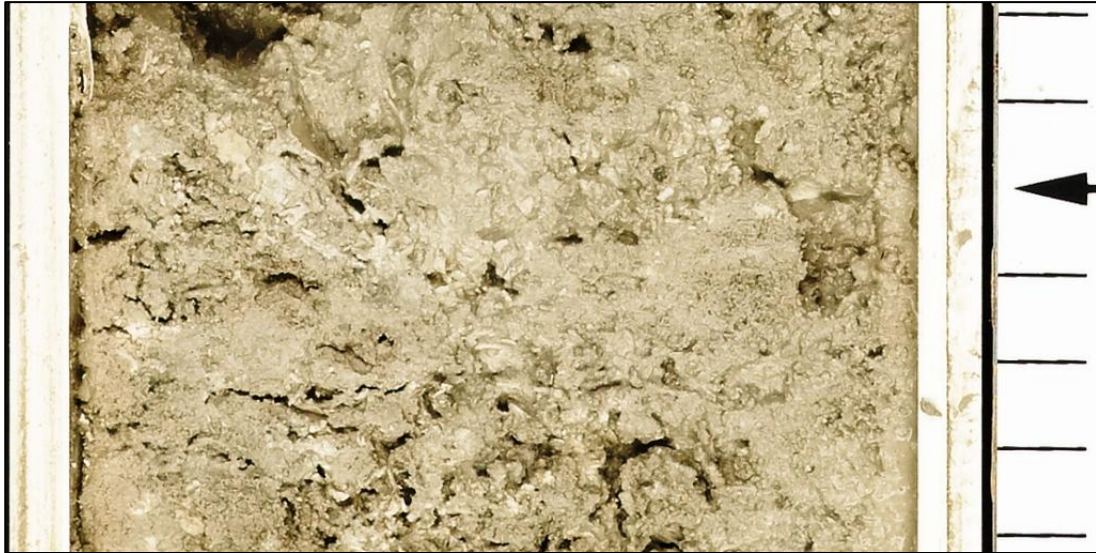
Fig 4.2.4: Coral-rich unit located at 180 cmdc (indicated by arrow head) in CS07 S2. This unit may explain the p-wave anomaly seen in the MSCL data at this level in Fig. 4.2.2. Each scale bar line represents one cm.
