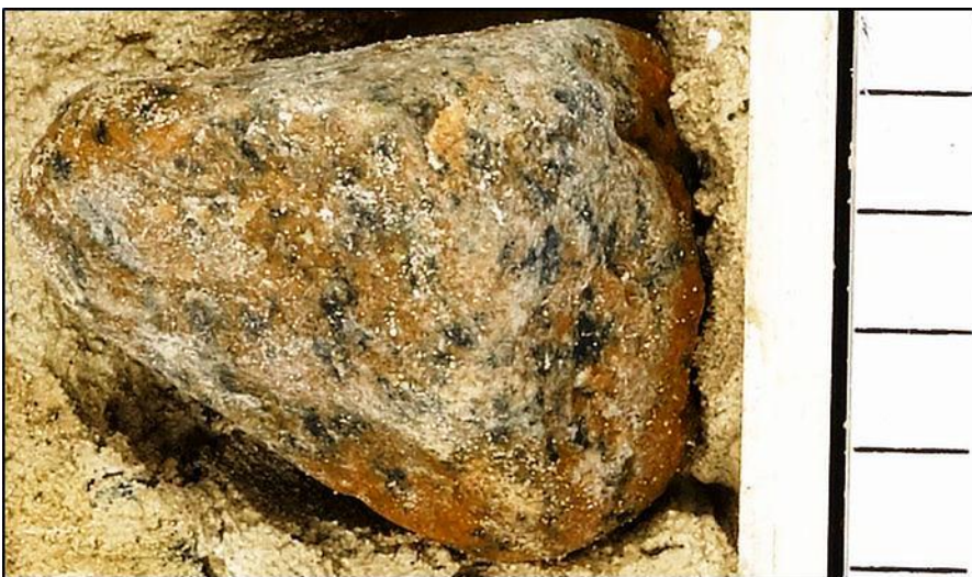
Fig. 4.6.7: Dropstone recovered from core CS06 Section 3, 235 - 239 cmdc, as pictured in-situ in the core. Scale of 1cm interval to the right
